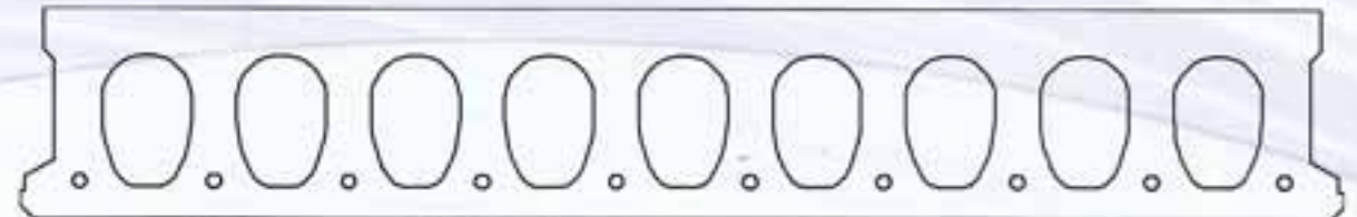
200mm thick slip-formed hollow core slab
