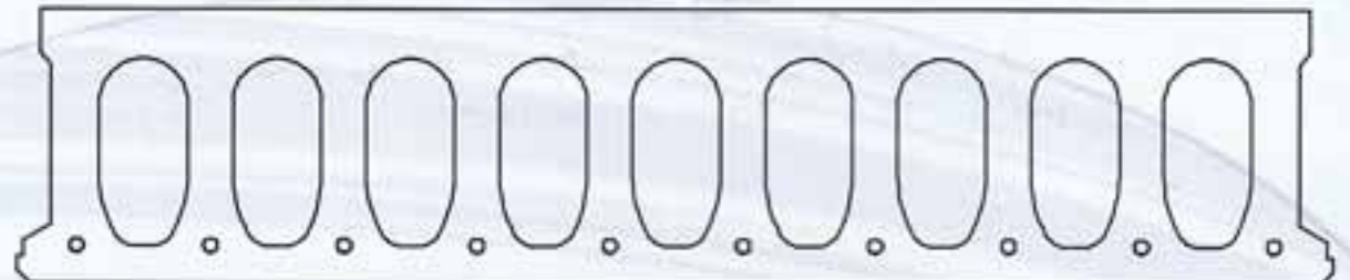
250mm thick slip-formed hollow core slab
